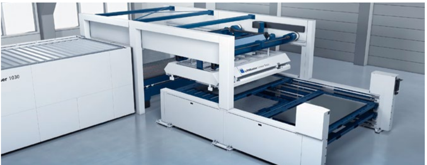
An introduction to automated manufacturing. Microstorage with automatic loading and unloading of the laser cutting machine at low investment costs.
