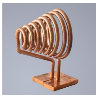
Sample parts printed with pure copper, like inductors, heat exchangers and electronics
