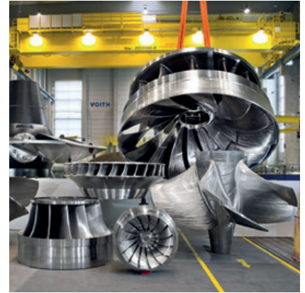
Turbines for hydro power generation Different components of hydropower equipment are produced in our high accuracy multitasking Vertical Lathes.
