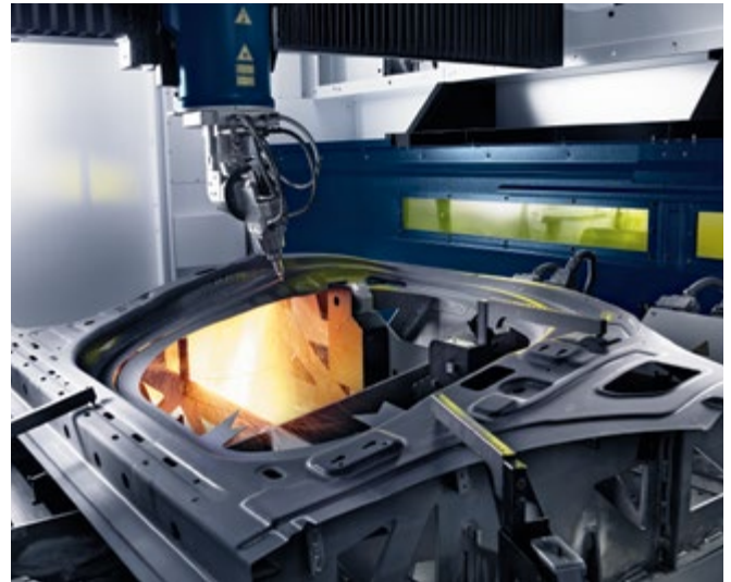
You can even process very large hot-formed parts with the TruLaser Cell 8030.
