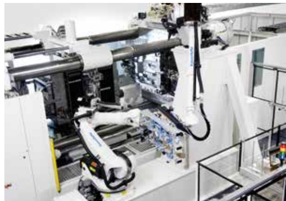
MX series designed as three-component SpinForm technology (swivel platen).
