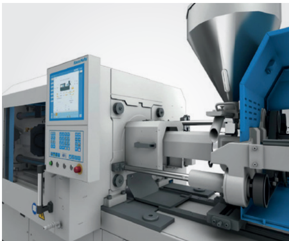
Injection unit movement via two parallel electric driven ball screws
