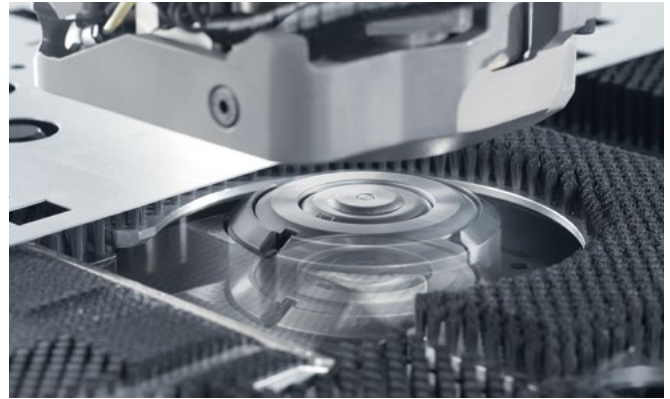
The descending die ensures scratch-free parts.
